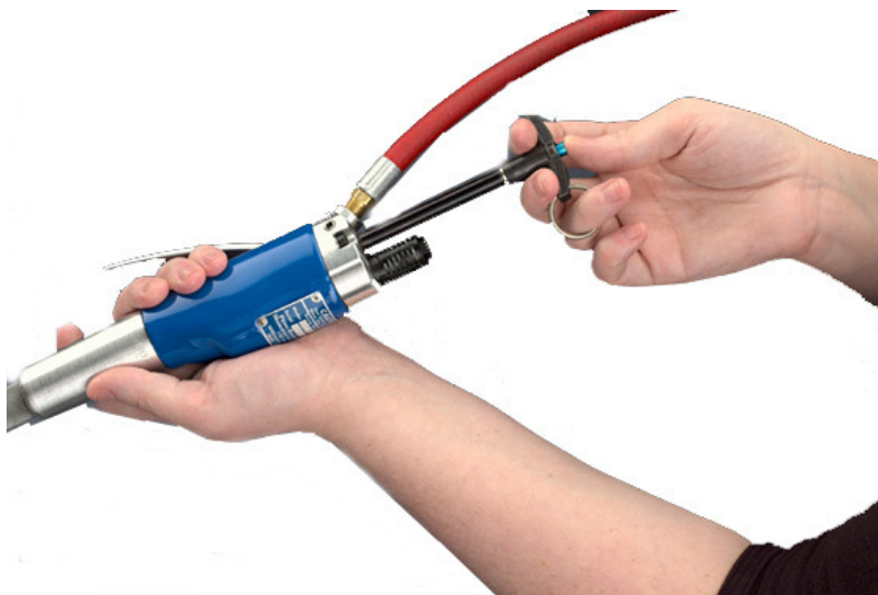
FIGURE 2 ADJUSTING TOOL STROKE FOR DIFFERENT LENGTH FASTENERS
