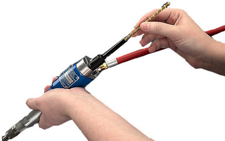
FIGURE 1 PROPER INSERTION OF STICK
