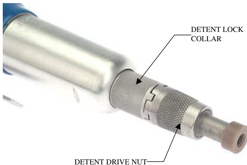
FIGURE 3 ADJUSTABLE LEVER NOSE ASSEMBLY
