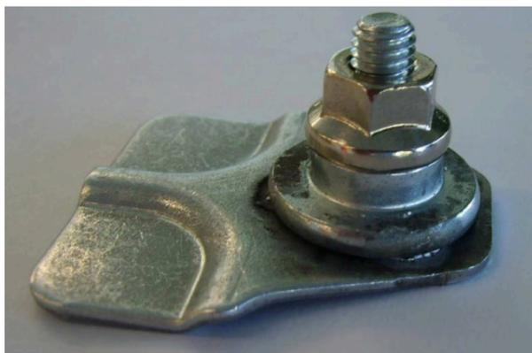
A classic solution of a welded earthing stud
