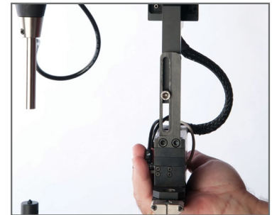
New T-bracket and shuttle with integrated connectors.
