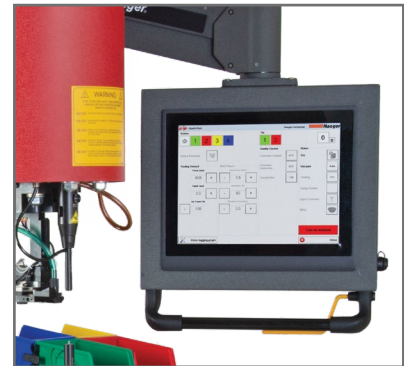
Operator control pendant adjustable in 6 directions.
