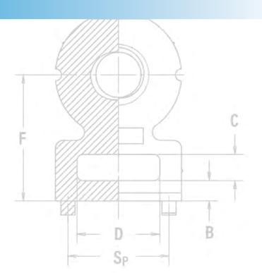
PEM® R'ANGLE® fasteners provide strong right angle attachment points in sheet metal or PC Boards. **RAA™** and **RAS™** fasteners for metal are simply pressed into a rectangular mounting hole of the proper size. **SMTRA™** fasteners are installed onto PC Boards using standard surface mount techniques. The holding power of the fastener is unaffected by the repeated tightening and loosening of the screw.
