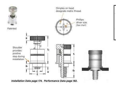
Threads: External, ASME B1.1, 2A / ASME B1.13M, 6g (1)
