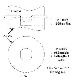
**NOTE:** The punch must be large enough to cover the entire base of the fastener to ensure proper installation.
