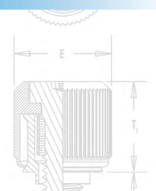
PEM® brand captive panel screws are designed to help keep parts to a minimum and eliminate risks associated with loose hardware that could fall out and damage internal components. These panel fastener assemblies are ideal to attach metal panels or other thin material components in applications where subsequent access will be necessary.
