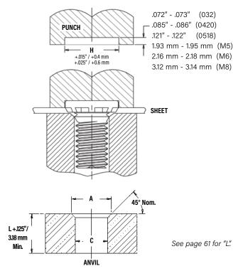
Tooling for sheet thicknesses .060" / 1.51 mm and greater with #10 / M5 and 1/4" / M6 thread sizes and .075" / 1.9 mm and greater with 5/16" / M8 threads.
