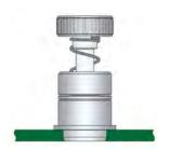
Installs in retracted/unfastened position
