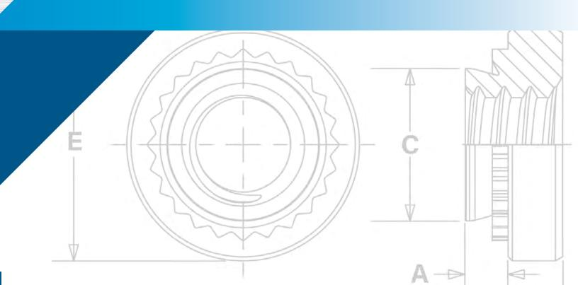
Self-clinching nuts are installed by placing them in properly sized holes in sheets and applying a parallel squeezing force to the head of the nut. The sheet metal surrounding the head cold flows into an undercut thereby making the fastener an integral part of the sheet. A serrated clinching ring prevents the fastener from rotating after installation.
