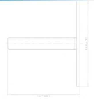
The PEM® VariMount® fastening system eliminates issues associated with welding. The assembly is comprised of a standard PEM® nut, stud or standoff mounted permanently into a base plate. The assembly can then be fastened or bonded to assorted panel types in a variety of ways:
