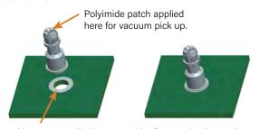
Solder paste applied to pad on PCB.
