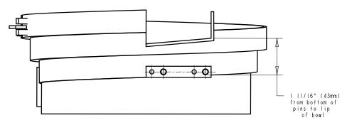
Bowl Dimension Check for use with special ramp escapements (Such as for middle dash length SO's and some R'Angle tooling packages).
