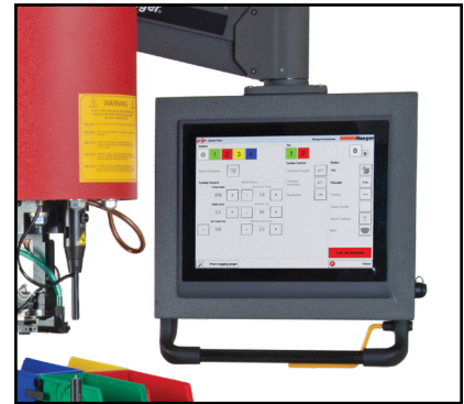
Operator control pendant adjustable in 6 directions.
