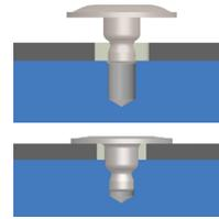
The Belleville shaped head flattens upon a simple press-in installation and draws panels together to accommodate vertical stack tolerances.
