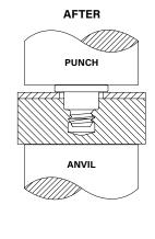
Shown with blind mounting hole. Can also be used with a through hole.
