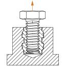
**Pullout** is the force required to pull the insert from the sheet.
