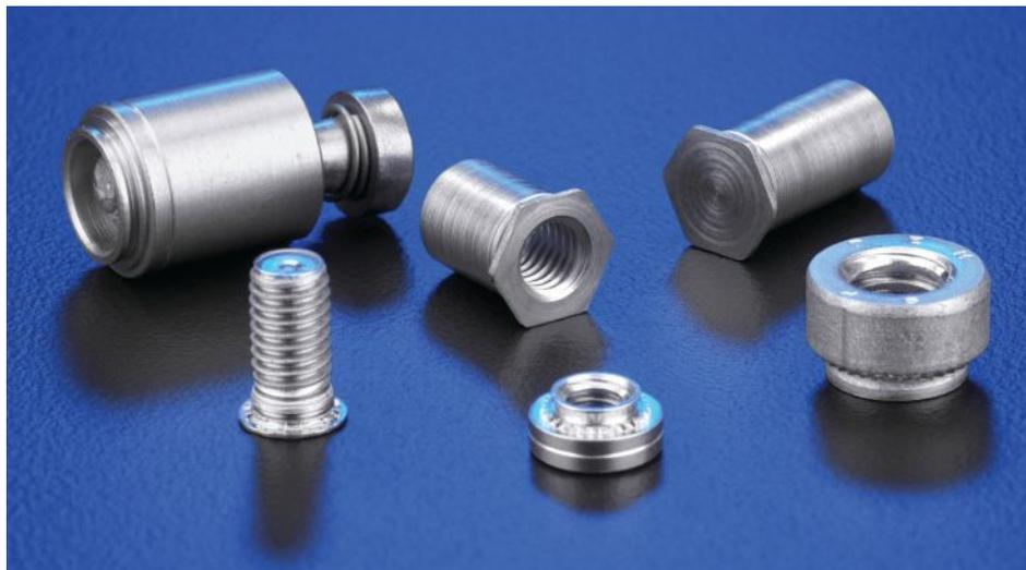
Due to the requirements of this process, the host metal sheet must always be sufficiently softer (typically 20 points on the HRB or HB hardness scales) than the fastener to prevent fastener deformation during installation. Sheets, too, must exhibit adequate ductility to allow the displaced sheet material to cold flow into the fastener's undercut without fracturing.
