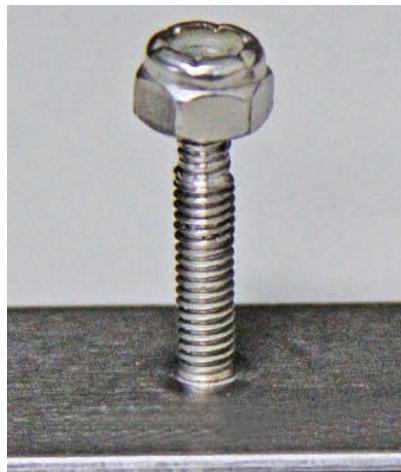
This installed self-clinching, flush-head stud with galled threads creates attachment difficulties with mating hardware (the nut at top).
