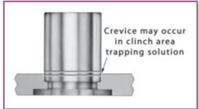
Figure 2. Illustration of a self-clinching standoff. Note the cavity beyond the fastener head.
