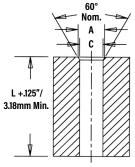
Recommended tooling when a chamfered anvil is required.
