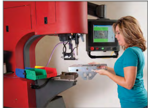
Operator control pendant adjustable in 6 directions.
