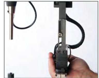
New T-bracket and shuttle with integrated connectors.
