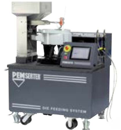
PEMSERTER® In-Die fastener feeding system.
