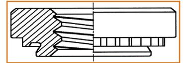
**For PEM® H and HNL nuts**, all of the above applies except the mounting hole tolerance which is greater at +.005. This yields .008" worst-case error.
