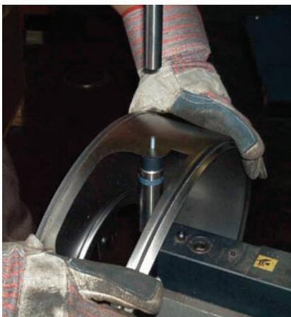
According to Austin Taylor, project engineer at A. O. Smith Water Products, an early plan was to utilize weld nuts on the water heater's round chamber ring. A mating screw then would be inserted through the access door.
