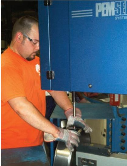
*Operator at A. O. Smith installs PEM studs in a combustion-chamber ring by utilizing a PEMSERTER Series 2000 press equipped with 'bottom-feed' stud tooling for the job.*
