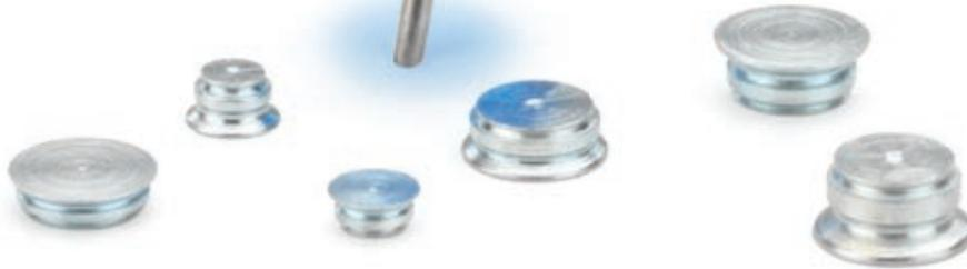
These unique fasteners permanently join two metal sheets to create a flush-attachment connection without protrusions on either side. They can serve as replacements for rivets or welding and their rotational capability extends application potential by enabling a single fastener to act as a hardened pivot point.
