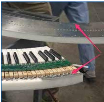
panels that compose the keyboard stands – creating load-bearing threads in the very thin sheets and providing high pushout and torque-out resistances. Mating screws complete attachment of units to stands.
