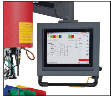
Operator control pendant adjustable in 6 directions.
