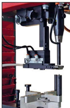
Multi-shuttle tooling platform for nuts studs and standoffs.
