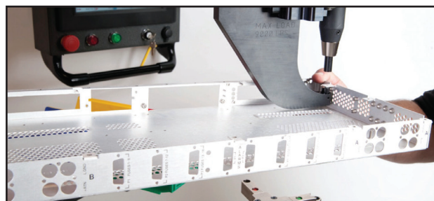
Manual J-Frame in combination with 24" (610mm) throat depth.
