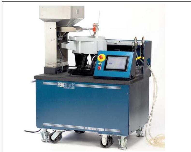
In terms of installation, once the die is completely built and in daily production, the stand-alone system can be hooked up within three to 10 minutes. Everything is quick-coupled and twistlock-connected.
