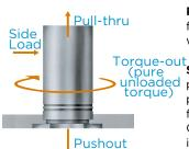
**Pull-through** – The resistance of a fastener to a force applied in the same direction to which it was installed.
