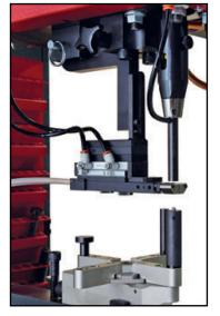
Multi-shuttle tooling platform for nuts studs and standoffs.
