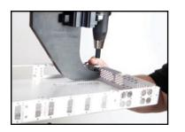
Manual tooling J-Frame is used for small boxes and short reverse flanges.
