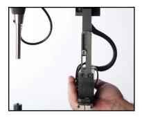
New T-bracket and shuttle with integrated connectors.
