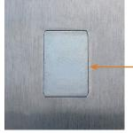
Depending on placement of the fastener within the mounting hole, on the reverse side of the sheet, a slight gap may be noticeable along the nonclinching edges of the fastener after installation. If gap is not acceptable in your application, check with techsupport for a solution.
