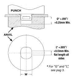
**NOTE:** The punch must be large enough to cover the entire base of the fastener to ensure proper installation.
