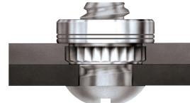
A [broaching fastener](#) is any knurled shank fastening device that is pressed into a prepared hole to provide a strong threaded attachment point in a non-ductile material.
